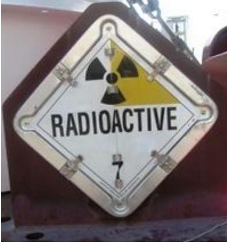
Interesting class 7 radioactive placard we have here!?! Where should the yellow triangle be and how big should it be? We are allowed to use hinged-type placards per 49 CFR 172.516(e) if the required format in 172.556 for a radioactive placard are maintained. Even if this is installed permanently on a trailer, who is at fault for allowing this placard to be used during transportation?
